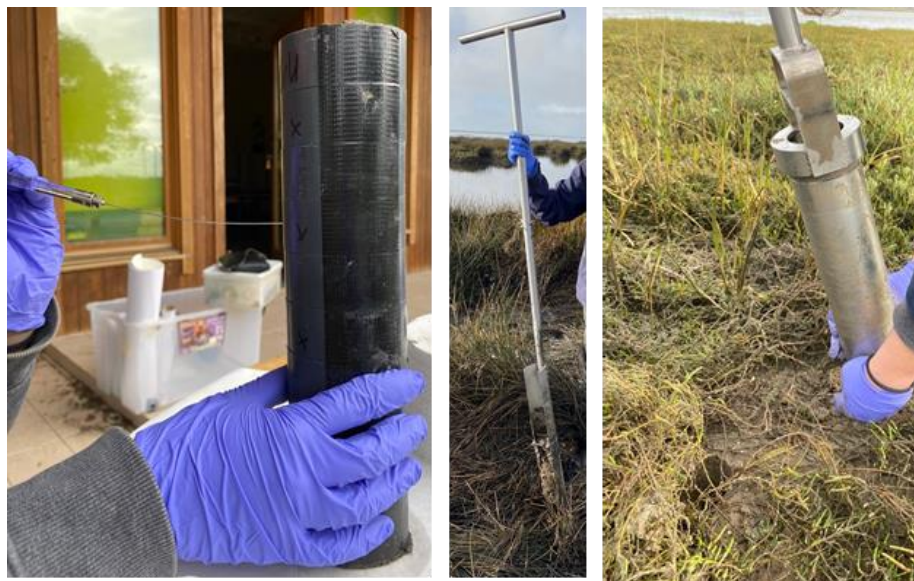
Figure 3 - (Right) Special metallic corer used to collect sediments for the isotope incubation experiment (Center) Metallic corer used to collect sediments for measuring physicochemical parameters, amount of biomass and content of metals (Left) injection of the isotopic solution in the inner PVC slices.
